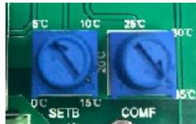
Variable resistors to set temperature
